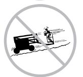
Limit travel speed according to the condition of the ground surface, congestion, slope, location of personnel, and any other factors which may cause collision.
