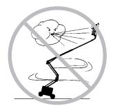
Do not raise the boom when wind speeds may exceed 12.5 m/s. If wind speeds exceed 12.5 m/s when the boom is raised, lower the boom and do not continue to operate the machine.
