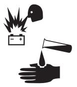
Batteries contain acid. Always wear protective clothing and eye wear when working with batteries.
