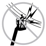
This machine is not electrically insulated and will not provide protection from contact with or proximity to electrical current.
